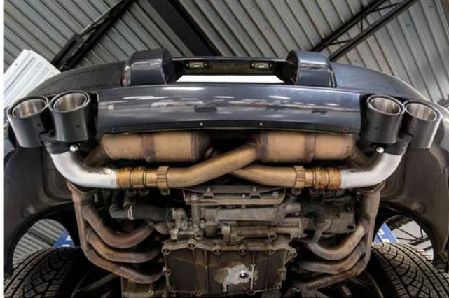
**Step 10:** Once final fitment is lined up, torque factory clamps and exhaust tip bolts. Enjoy your new muffler bypass pipe!
