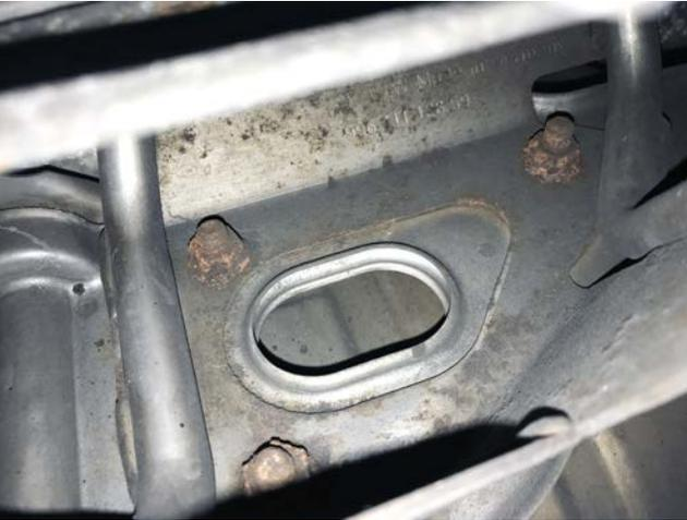
**Step 6:** Remove 3 x 13mm muffler support bracket nuts.
