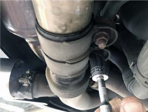
**Step 2:** Loosen 13mm sliding exhaust clamp bolts.
