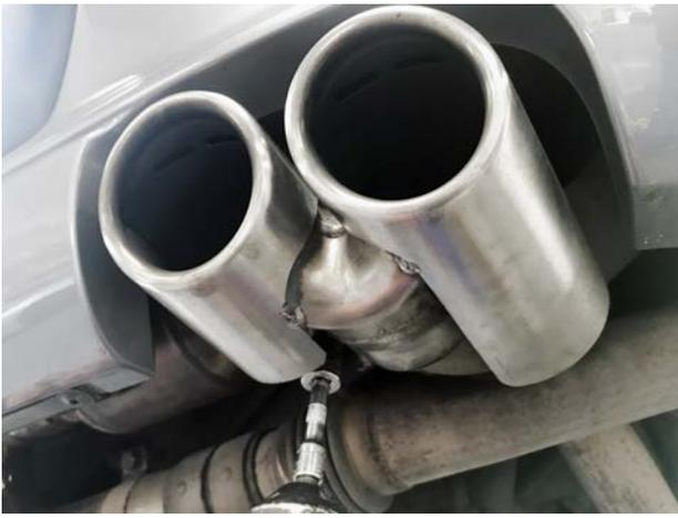
**Step 1:** With the rear of the vehicle raised and supported safely, locate the 13mm exhaust tip mounting bolts and loosen. Slide the exhaust tips off of the vehicle.
