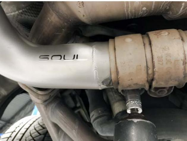
**Step 8:** Slide the SOUL muffler bypass pipes into the factory clamps and tighten just enough to allow for final adjustment after tips are installed
