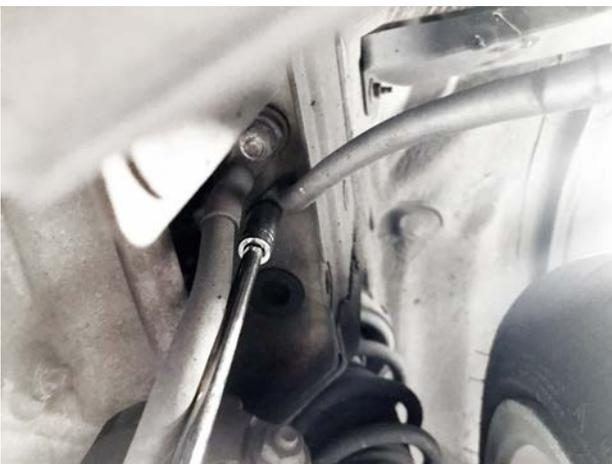
**Step 4:** Remove 10mm bolt from bumper support rod.
