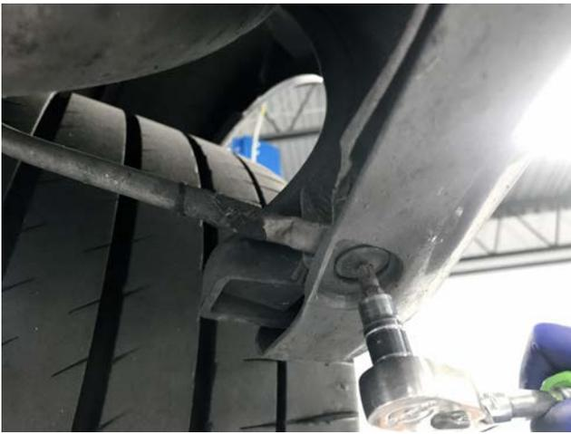
**Step 5:** Remove T30 bolt from other side of the bumper support rod.
