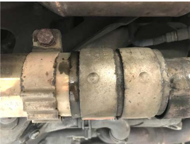
**Step 3:** Slide clamps off the mufflers and onto the catalytic converter sections.
