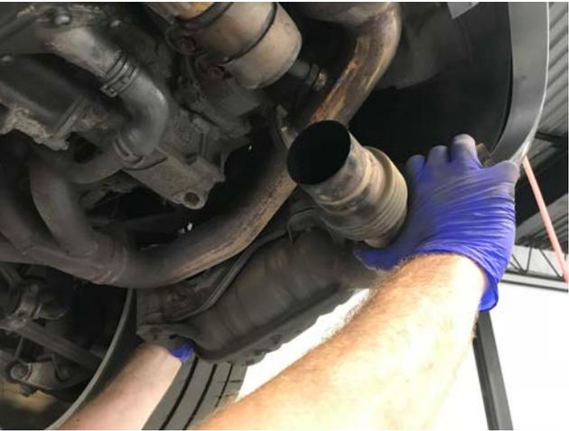
**Step 7:** Remove the OEM mufflers from the vehicle.
