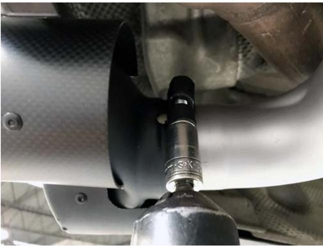
**Step 9:** Loosely install factory / SOUL exhaust tips. Line up muffler bypass piping and tips to be suitable for placement in the bumper.
