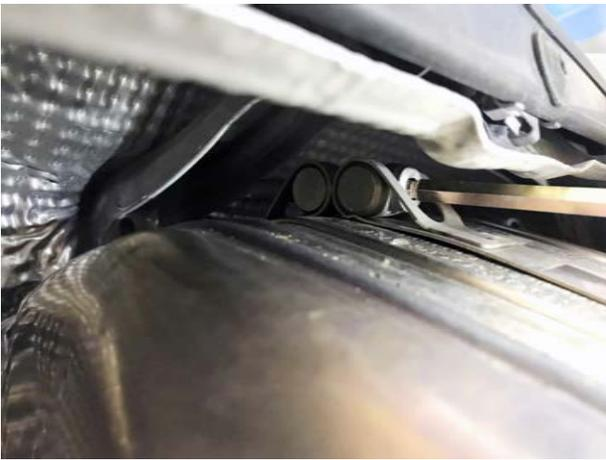
**Pictured Left:** Loosen the muffler band straps using a 6mm allen key. Loosen them enough to allow movement of the rear muffler to aid in the removal of the headers.
