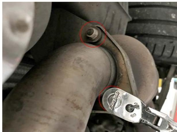
**Pictured Left:** Remove the 13mm nuts from the header/muffler flange.
