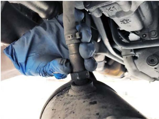
**Pictured Left:** You can now remove the oxygen sensors, taking note of their correct orientation and position.
