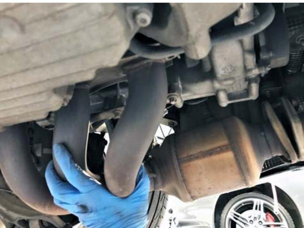
**Pictured Left:** Carefully guide your OEM headers down and out of the car.
