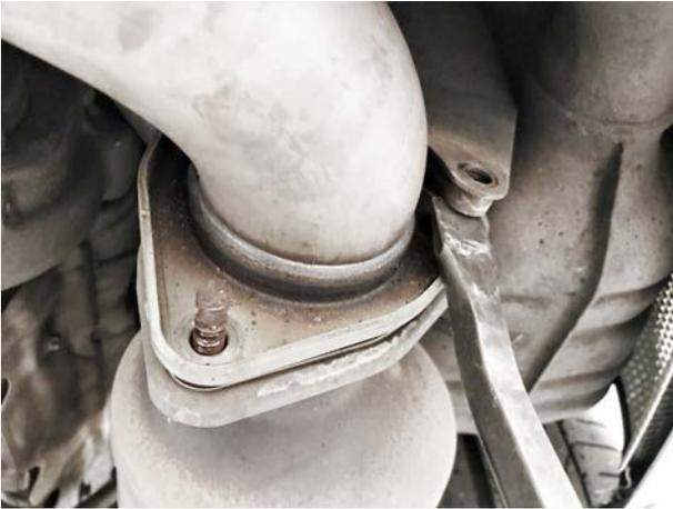
**Pictured Left:** You may need to pry the support bracket for the side mufflers off of the studs on your factory headers. Utilize the movement gained by loosening the rear muffler band straps to aid in this process.
