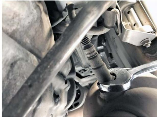
**Pictured Left:** Carefully use your 22mm wrench to loosen (**do not fully remove**) the oxygen sensors, there are two per side. It is imperative that the oxygen sensor locations do not get mixed up on re-installation. You can mark them as fore and aft to help avoid confusion.
