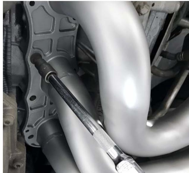
**Pictured Left:** Using your E-12 torx socket, loosely tighten the remaining hardware to the same depth.
