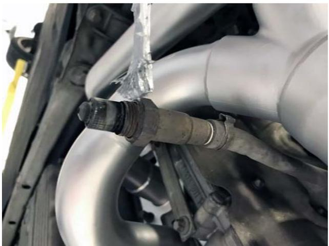
**Pictured Left:** Coat the threads of the oxygen sensors with anti-seize to make future removal easier.
