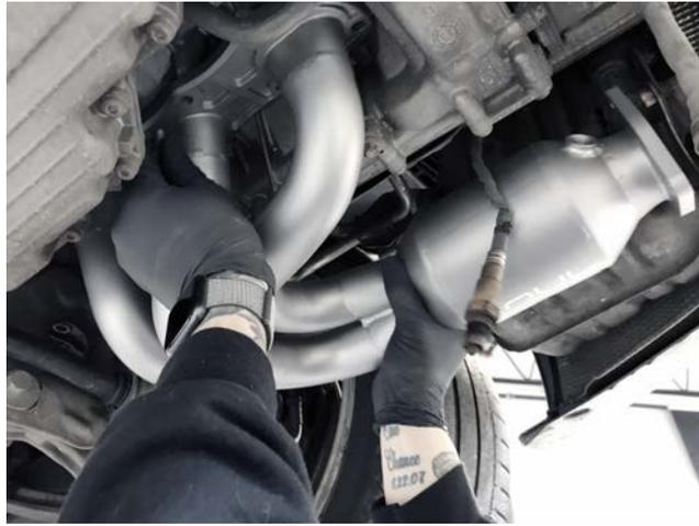
**Pictured Left:** Guide your new Soul Performance headers into place and loosely tighten the hardware.
