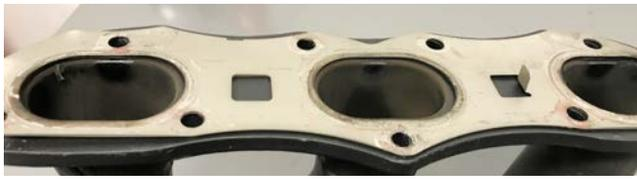
**Pictured Left:** Coat your OEM gaskets with a copper gasket sealant and install onto your Soul Performance headers with the tab in the vertical position as shown.
