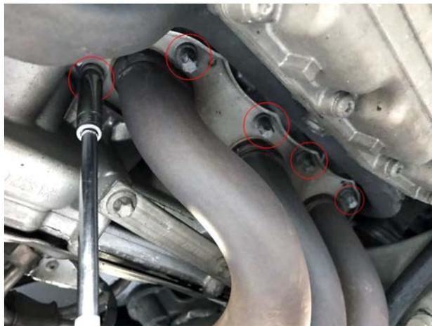
**Pictured Left:** Using the E-12 torx socket, remove the 9 bolts per side holding the headers to the cylinder head.
