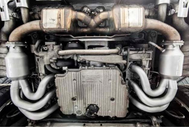
**Pictured Above:** Completed installation of Soul Performance Products Long Tube Street Headers
