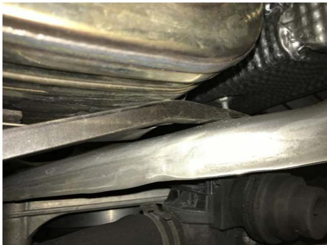
**Pictured Left:** You may need to pry between the muffler can and the muffler mounting bracket in order to move the rear system into alignment with the header flanges. This is why we loosened the band straps in step 2.
