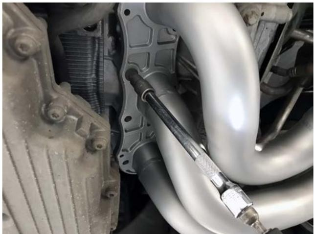
**Pictured Left:** Tighten the E-12 Torx bolts to specification, starting from the outside and working your way in to the middle.
