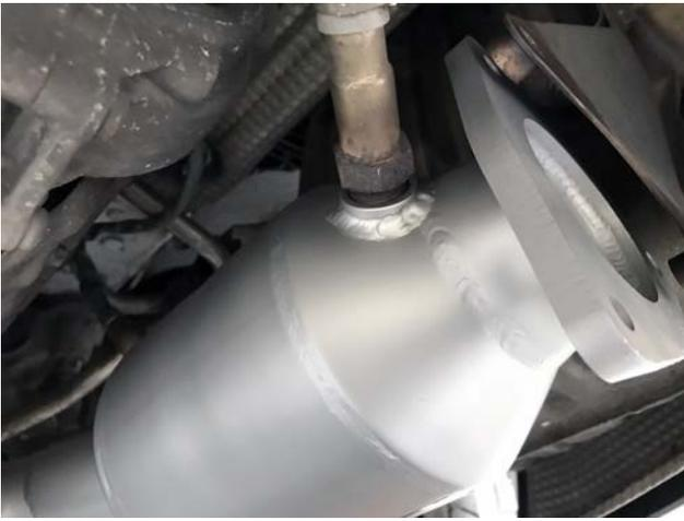
**Pictured Left:** Install oxygen sensors into their correct positions and tighten using 22mm wrench.
