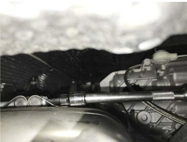
**Step 3B:** Loosen both driver and passenger straps but do not yet remove the 6mm allen bolt on them.
