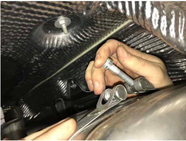
**Step 3C:** Each bolt can now be swung free to release band straps - remove them.
