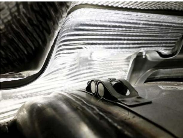
**Step 3A:** Locate the OEM band straps holding up the muffler on both the passenger and driver side.
