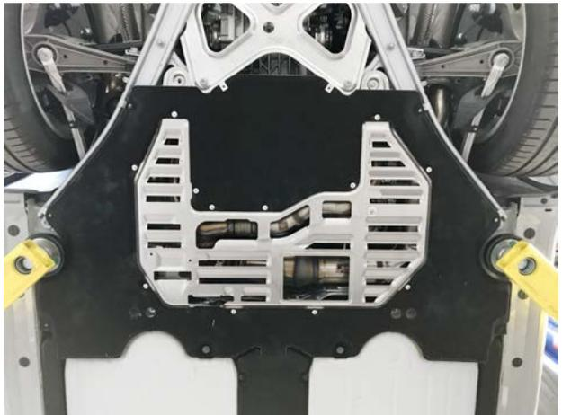
**Step 7:** Remove chassis braces to give better access to downpipe. (16mm nuts)
