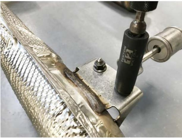
**Step 8:** Remove exhaust hanger (12mm nuts) from OEM Y pipe.
