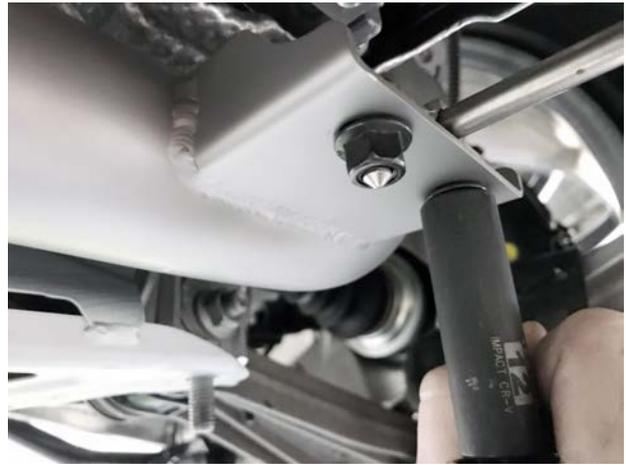
**Step 14:** Tighten exhaust hanger nuts to 12-15 Ft LBS.
