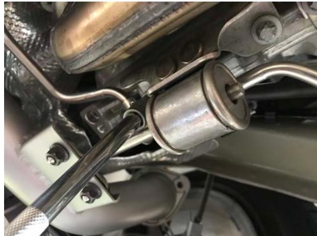
**Step 12:** Install exhaust bracket, torque to 15-18 Ft LBS.
