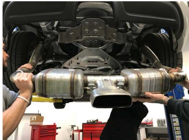
**Step 5:** The OEM muffler can now be removed from the vehicle. We recommend two sets of hands or the use of a jack to support the weight of the muffler as it is quite heavy.
