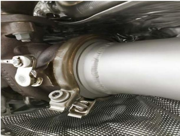
**Step 10:** Make sure the turbo and downpipe mating flanges are seated properly and install the OEM clamp on the cat section (with 90 degree bend section attached).
