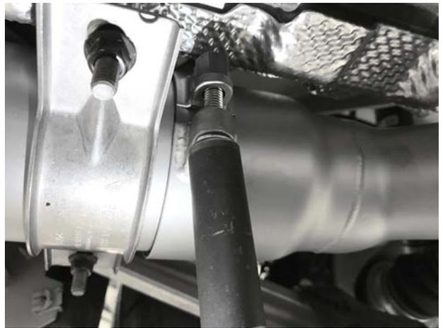
**Step 17:** Now that all downpipe clamps are in place and torqued down, replace and tighten chassis braces to 40-45 ftlbs .
