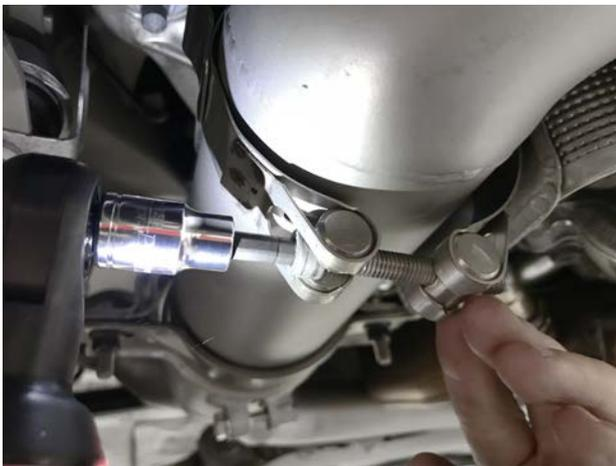
**Step 15:** Fully tighten OEM band strap onto the 90 degree downpipe section.
