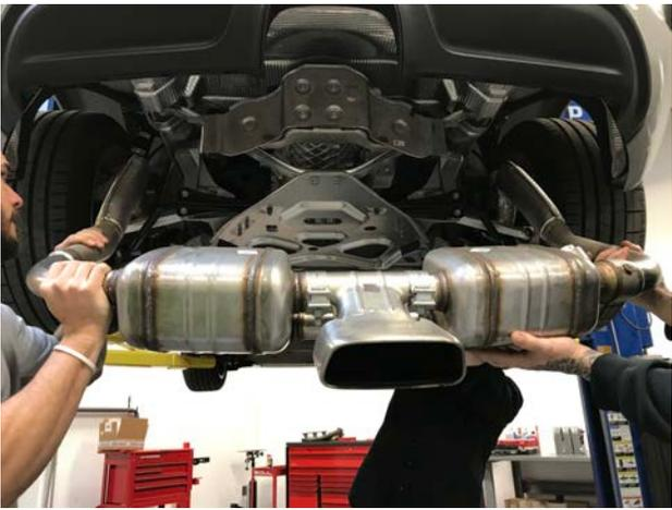
**Step 18:** Reinstall belly pan and exhaust following the reverse procedure of installation.
