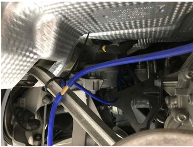
Pictured Right: Safely route vacuum lines as shown and down to exhaust valves (shown without exhaust for better visibility).
