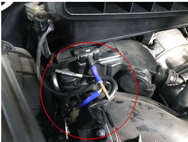
Pictured Right: Unhook and remove vacuum line from T-fitting to solenoid as pictured.
