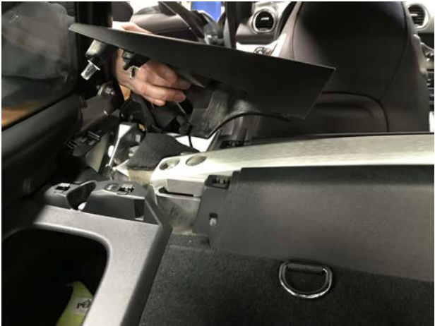
Pictured Left: Remove Torx bolts holding on brace
