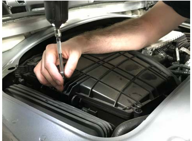
Pictured Left: Completely remove airbox to allow for better access
