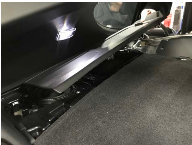
Pictured Right: Remove Torx screws holding in rear plastic
