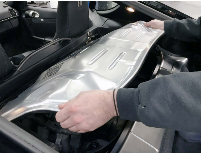
Pictured Left: Remove the engine compartment lid
