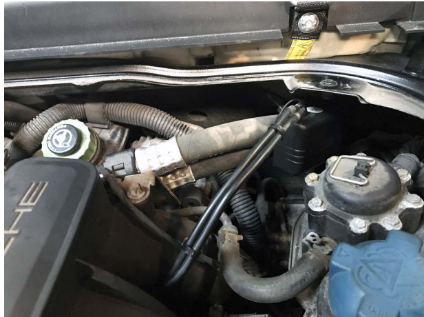
Pictured Left: Neat installation with proper cable management
