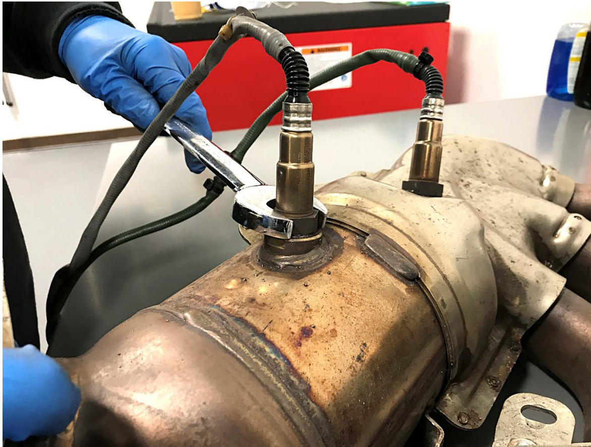
Pictured Left: Carefully remove both oxygen sensors from your factory headers. Depending on the age/usage of your vehicle this may take some patience/heat. The o2 Sensor Bungs are 22mm.
