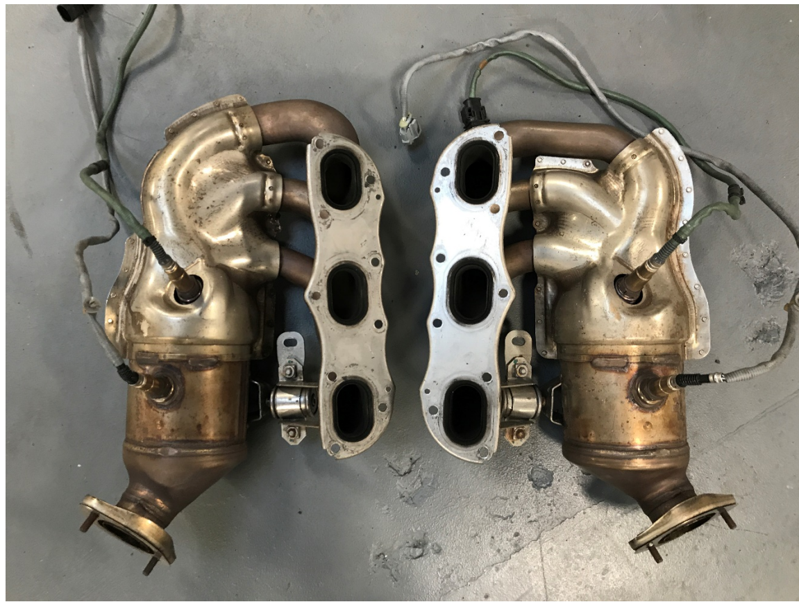
Pictured Left: Carefully remove the factory headers to avoid damaging the oxygen sensors
