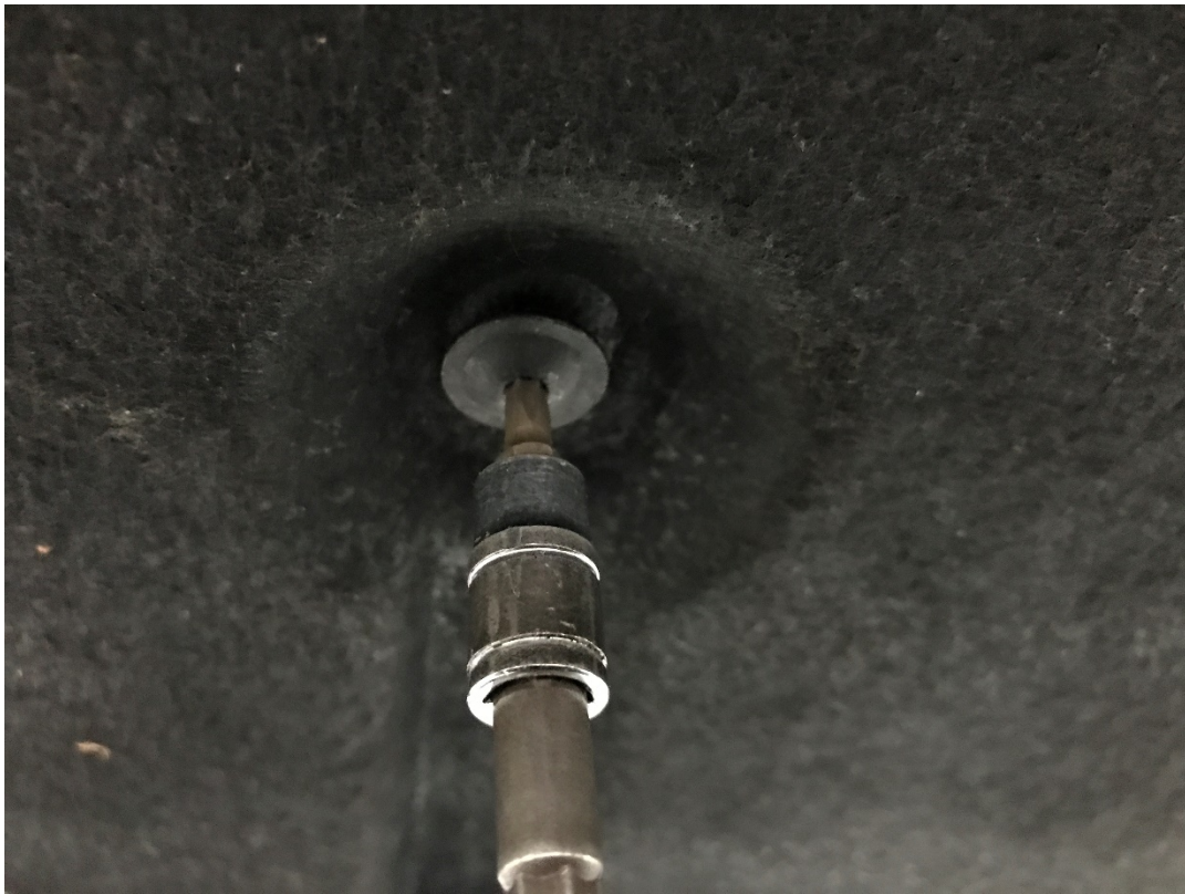
Pictured Left: Remove the under body panels by undoing the four 10mm bolts and five T-25 Torx bolts
