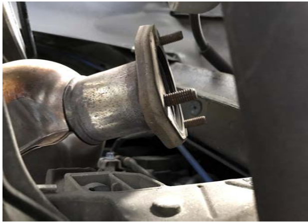
Pictured Right: Tighten down bolt with 13mm wrench.
