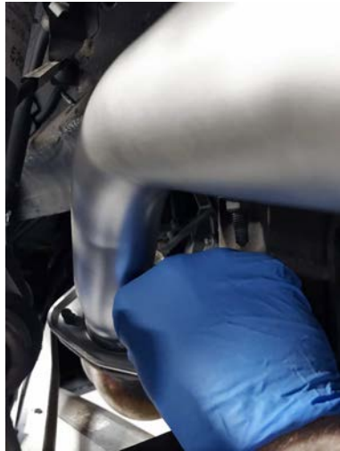
Pictured Left: Slide the driver's side half of your new SOUL exhaust up and into its position. Loosely tighten the three 13mm supplied nuts onto the header flanges enough to provide support but still loose enough to allow for adjustment later.
