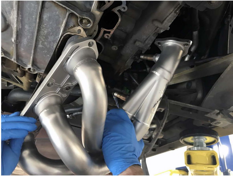
Pictured Left: Guide your SOUL headers back into place following the reverse sequence of removal.
