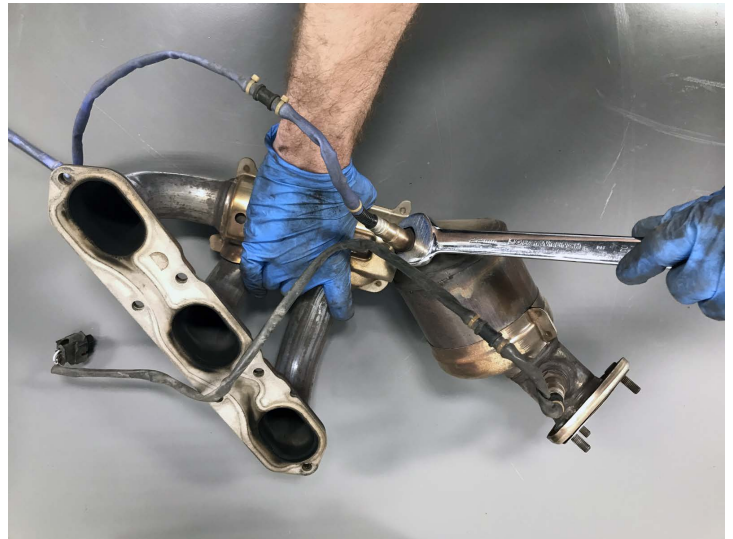
Pictured Left: Remove the 13mm bolts from the header flanges. There are six per side, you will be re-using these.
