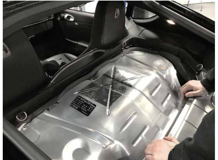
Pictured Right: Remove the engine compartment lid by taking out the mounting hardware. In this case, there were 5 torx bolts holding it in place.
