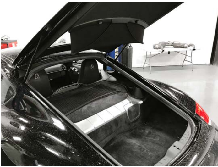
Pictured Left: Gain access to the engine compartment of your car. In this case on the Cayman, lift the rear hatch and remove the carpeting above the engine.
