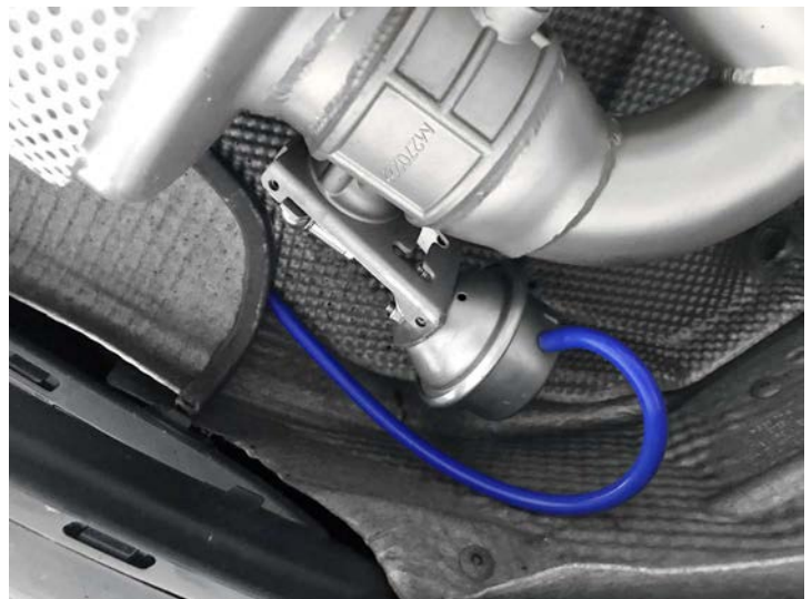
Pictured Right: The newly run vacuum line attached to the valve on your new Soul Performance Products Exhaust. We chose to tuck our vacuum tubing behind the factory heat shields, you can do it this way or another way of your choosing.
