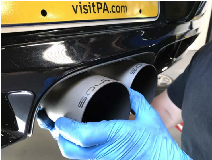
Pictured Left: Reinstall SOUL exhaust tips, set the depth and tighten the tip clamps to a minimum of 40 ft-lbs (13mm)
