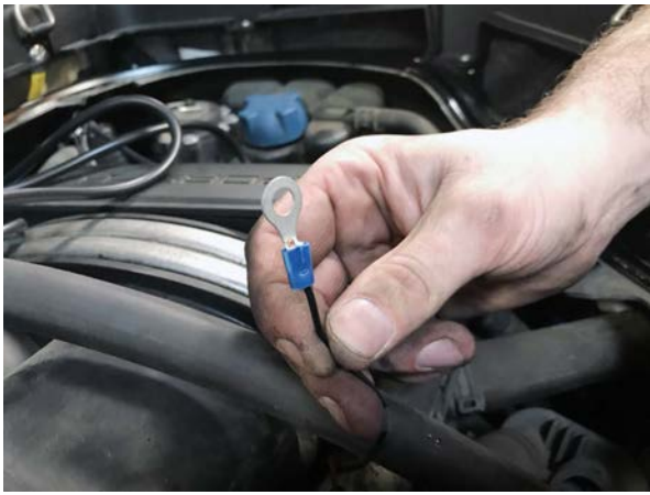
Pictured Right: Attach the ground to the engine or frame of the car. Make sure that the connection point is clear of any rust or grease.
