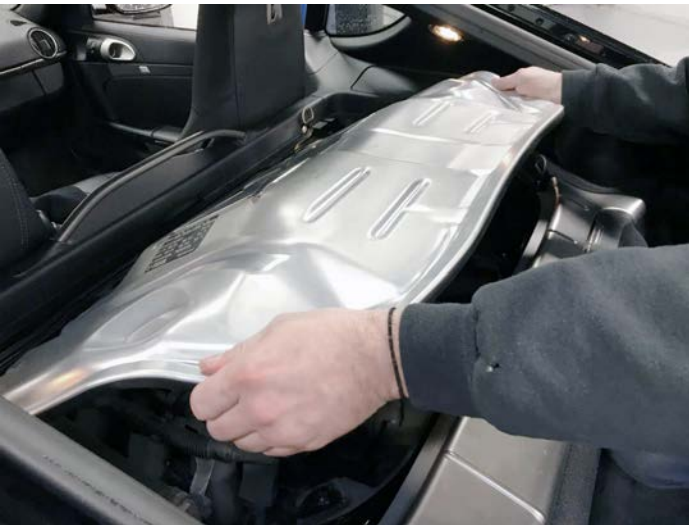
Pictured Left: Remove the engine compartment lid
