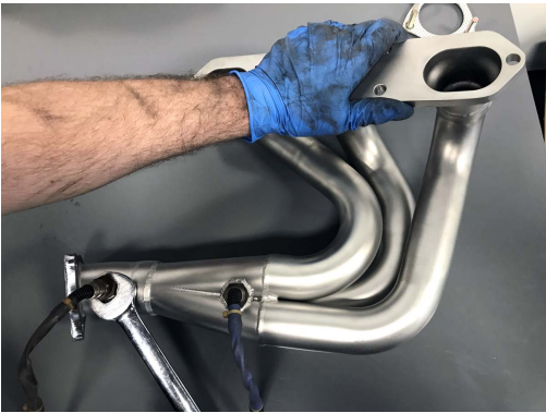
Pictured Left: Install the oxygen sensors into their respective positions and torque to 37 - 44 ft-lb.
