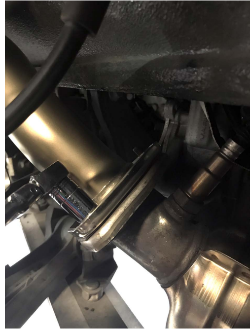
Pictured Left: Locate the oxygen sensor wiring mounting locations and disconnect/remove the sensor clips and tie downs.
