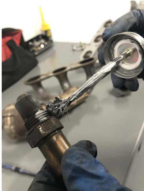
Pictured Left: Install the oxygen sensors into their respective positions and torque to 37 - 44 ft-lb.
