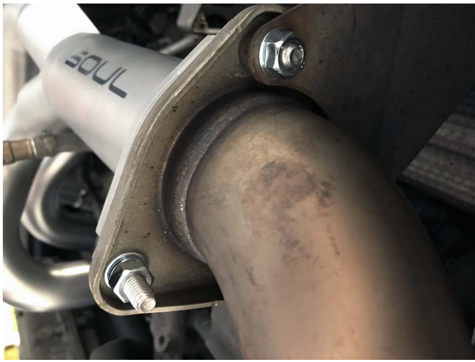
Pictured Right: Using your E-12 torx socket, loosely tighten the remaining hardware to the same depth.
