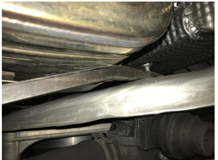
Pictured Left: With the header flange, muffler flange and side muffler support bracket in line, install and snug the hardware. The M8-1.25x40mm bolts/washers go into the top two positions where the side muffler bracket mounts and the M8-1.25x30mm bolt/washer goes in the remaining location at the bottom of the flange.
