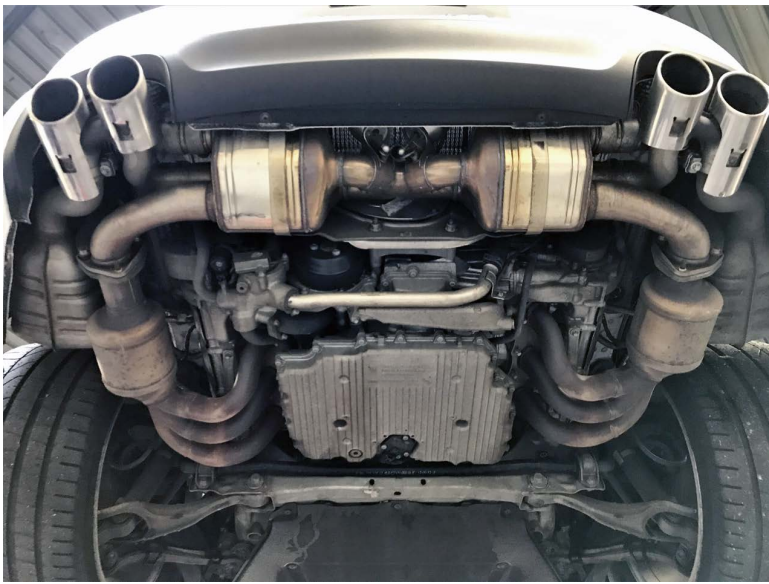
Pictured Right: Carefully use your 22mm wrench to loosen (do not fully remove) the oxygen sensors, there are two per side. It is imperative that the oxygen sensor locations do not get mixed up on re-installation. You can mark them as fore and aft to help avoid confusion. Take precaution as to not damage the wiring.
