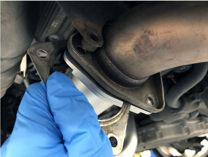
Pictured Right: You may need to pry between the muffler can and the muffler mounting bracket in order to move the rear system into alignment with the header flanges. This is why we loosened the band straps in step 2.
