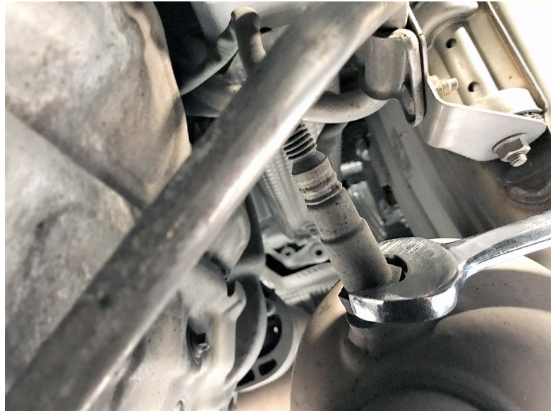
Pictured Right: Carefully use your 22mm wrench to loosen (do not fully remove) the oxygen sensors, there are two per side. It is imperative that the oxygen sensor locations do not get mixed up on re-installation. You can mark them as fore and aft to help avoid confusion. Take precaution as to not damage the wiring.
