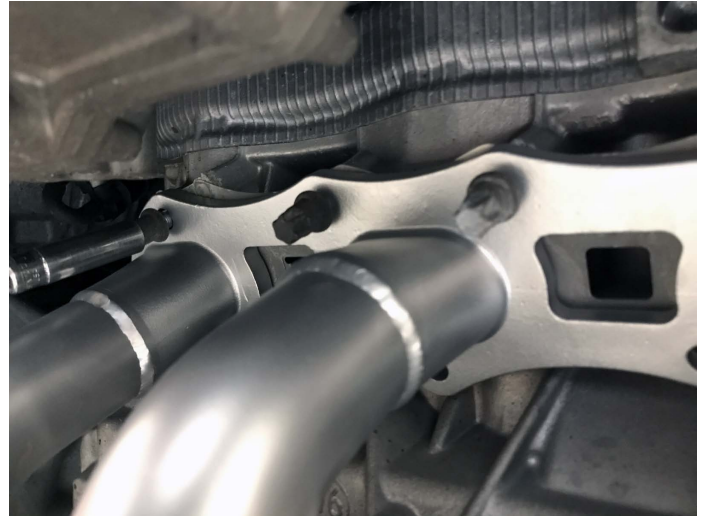
Pictured Left: Coat the OEM gaskets in a copper gasket sealant and guide them into place. You can slide on of the bolts into position (without the nut) to hold it in place if needed.
