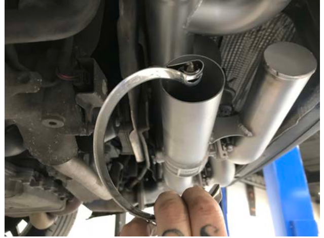
Pictured Left: Tighten factory clamp connecting factory side mufflers to SOUL exhaust
