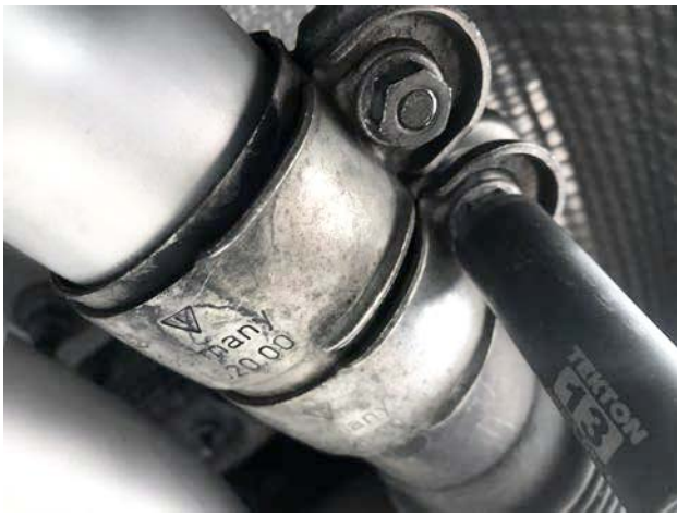
Pictured Right: Stretch Mikalon clamps to go over factory mounting brackets and SOUL X-pipe
