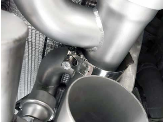
Pictured Right: Stretch Mikalon clamps to go over factory mounting brackets and SOUL X-pipe
