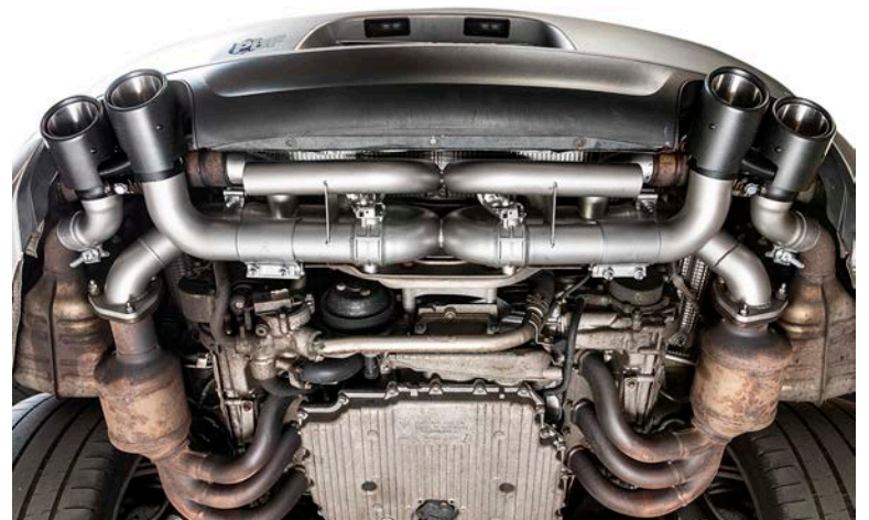
Pictured Above: Tighten all clamps, Torca clamps down (45 ft-lbs)
