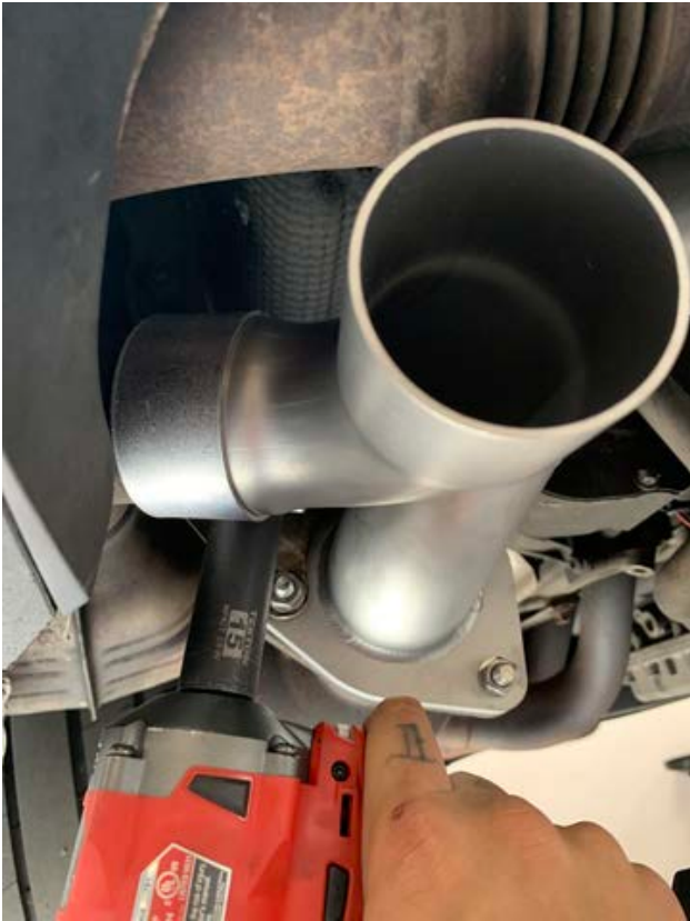
Pictured Right: Adjust the tip tubes and tubes coming off the exhaust to align inside the tips and tighten down the tips onto the tip tubes.
