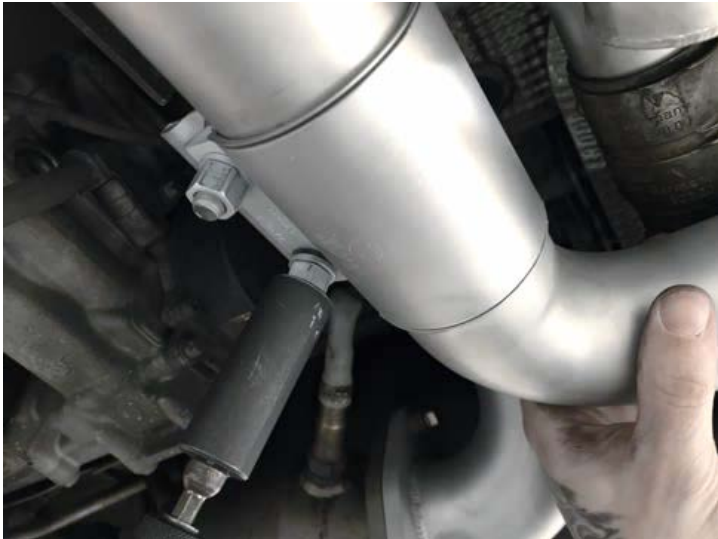
Pictured Above: Tighten all clamps, Torca clamps down (45 ft-lbs)
