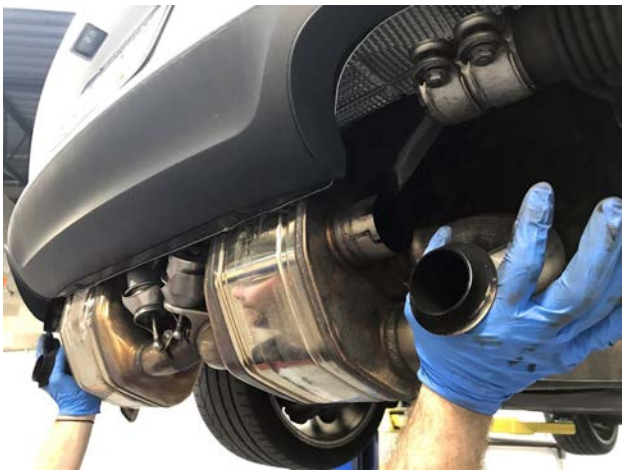
Pictured Right / Below: There is 3" of straight piping on the factory mufflers. Measure out the 3" and mark 1.6" in. This is where you will need to cut. Cut cleanly and remove all burrs and imperfections for a clean installation. DO NOT COMPLETE THIS STEP ON A "S" NON-PSE CAR.
