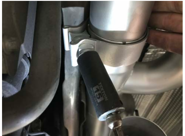
Pictured Left: Tighten factory clamp connecting factory side mufflers to SOUL exhaust
