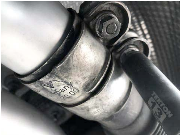
Pictured Right: Stretch Mikalor clamps to go over factory mounting brackets and SOUL X-pipe
