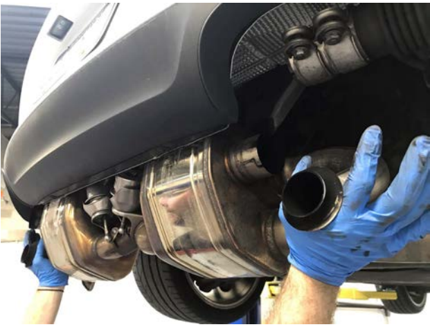
Pictured Right: Install inlet pipes loosely with AccuSeal clamps onto X-Pipe section.
