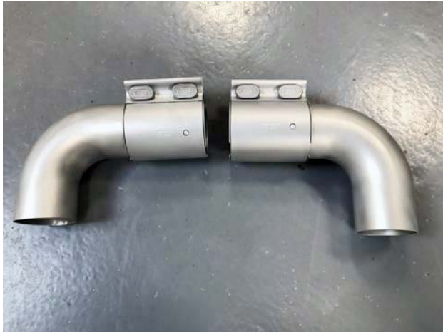
Pictured Right: Loosely install outlet section onto SOUL X-pipe
