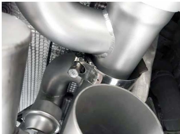
Pictured Right: Stretch Mikalor clamps to go over factory mounting brackets and SOUL X-pipe
