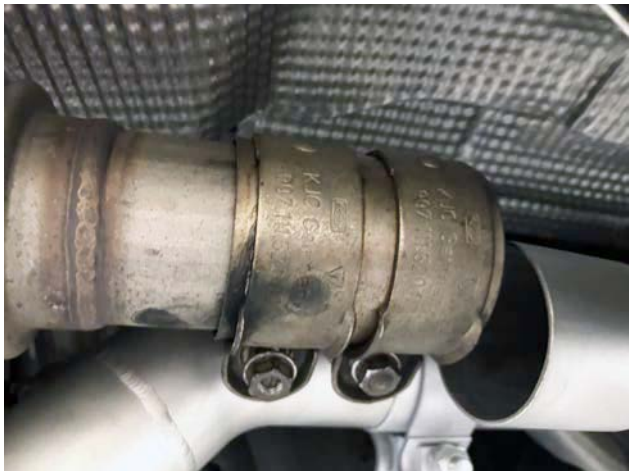
Pictured Right: Loosely install gaskets and supplied 13mm hardware.
