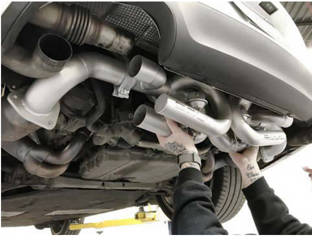
Pictured Right: Loosely install gaskets and supplied 13mm hardware.
