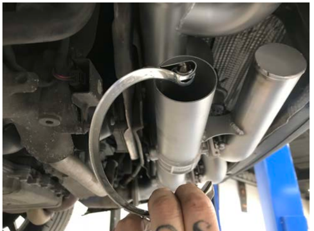
Pictured Left: Tighten factory clamp connecting factory side mufflers to SOUL exhaust
