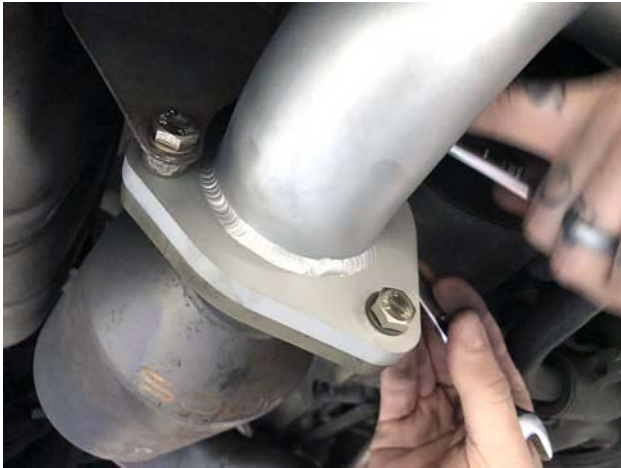
Pictured Right: Torque down AccuSeals holding X-Pipe to inlets
