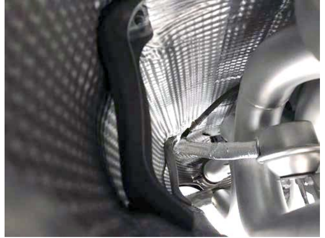
Pictured Left: Loosely install Torca clamps onto outlet pipes. (15mm nuts)
