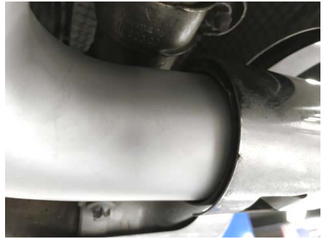
Pictured Left: Install, position, and tighten down tips.
