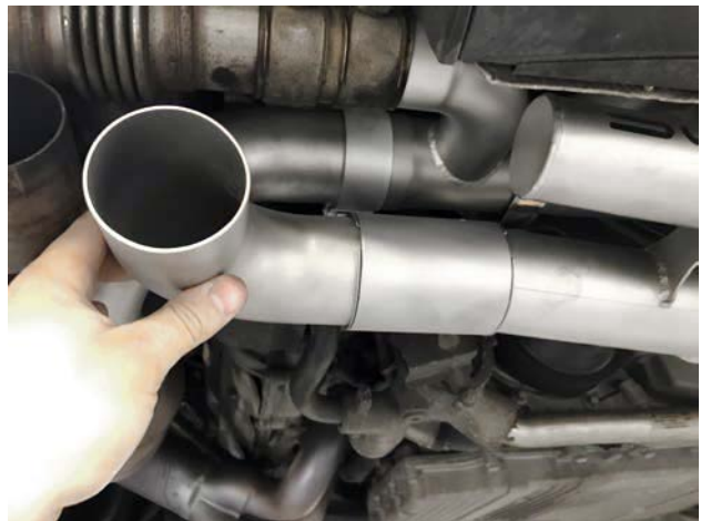
Pictured Left: Loosely install Torca clamps onto outlet pipes. (15mm nuts)
