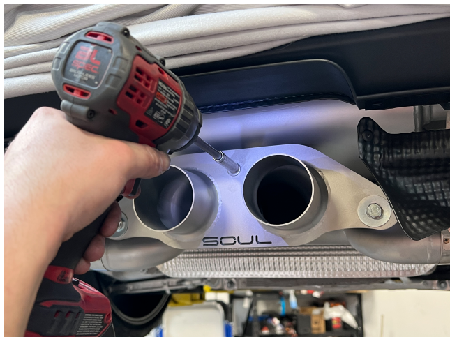
Step 14: Secure tip plate with provided gasket onto center muffler plate.
