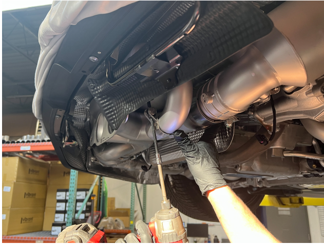
Step 11: With side connections still loose, securely fasten center muffler section band clamps.
