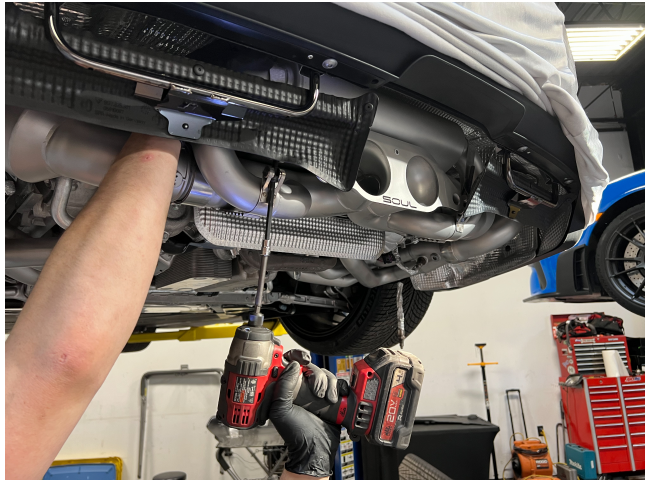
Step 12: Securely fasten all four Accuseal clamps on muffler inlet and outlet pipes.
