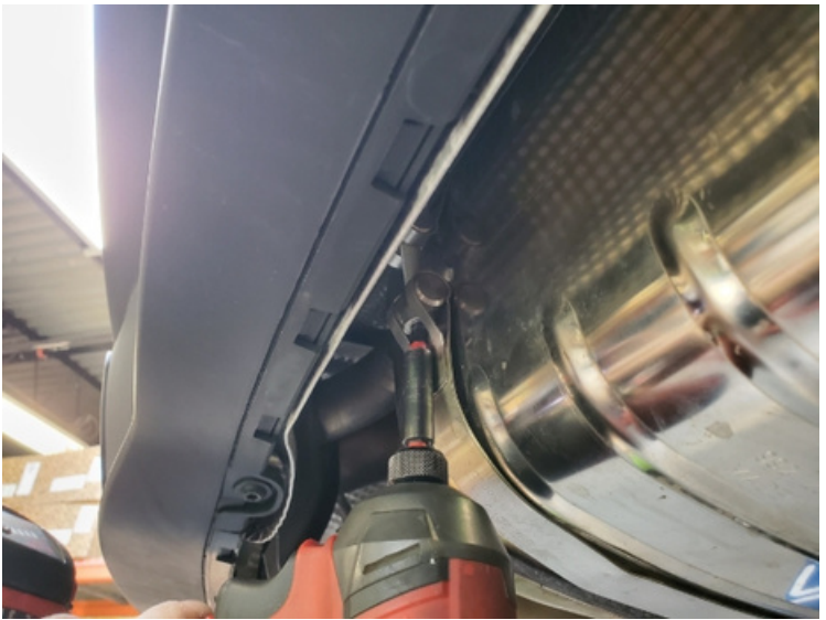
Step 18: Fully tighten the clamps between the muffler and catalytic converters.(13mm)
