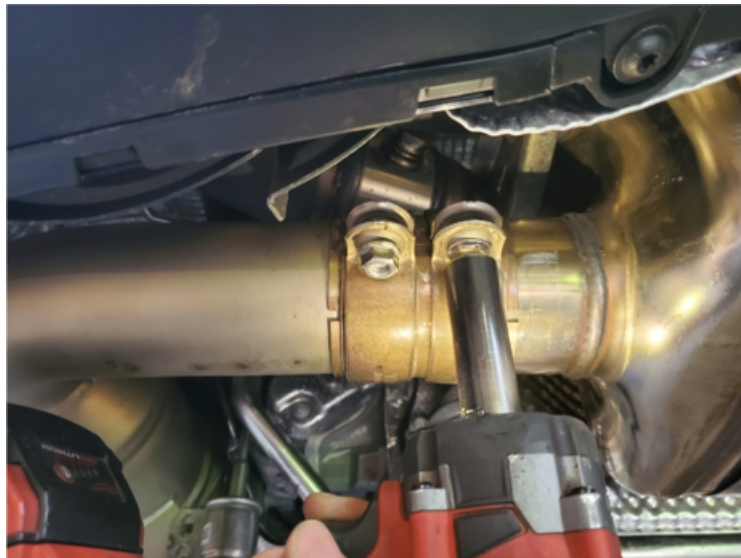
Step 17: Fully tighten the muffler straps
