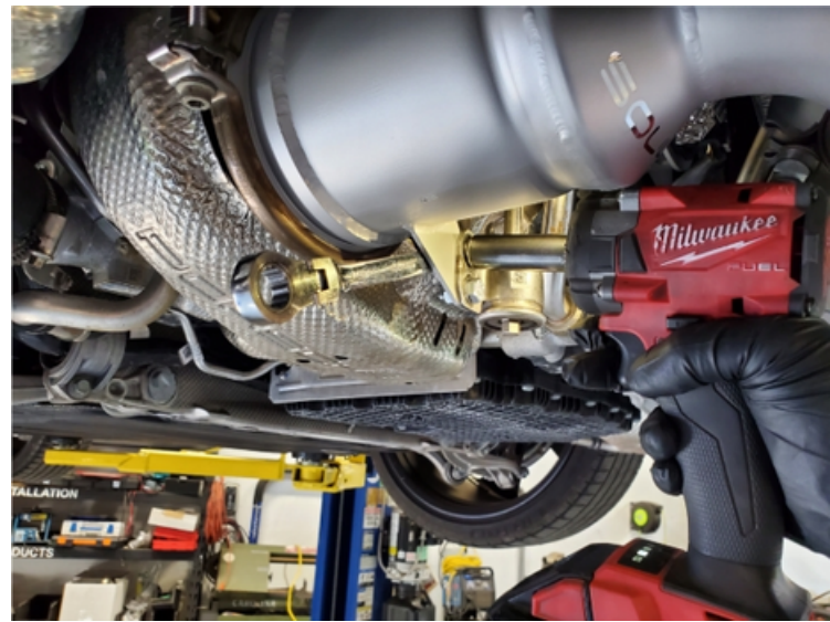
Step 49: Fully Tighten the clamps onto the turbos with a 6mm Allen socket
