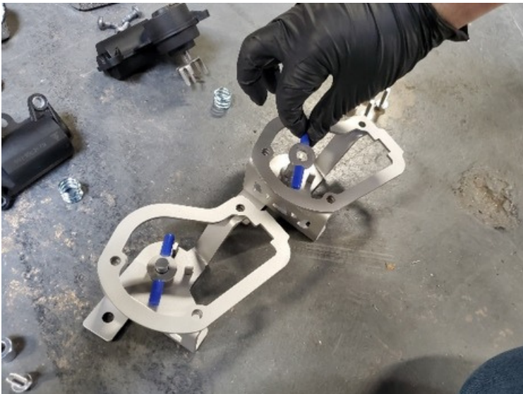
Step 17: Install The 3/4" diameter aluminum spacers to the pins on the brackets.
