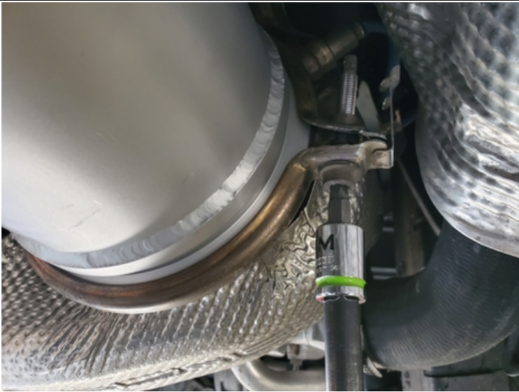
Step 50: Tighten the brackets on the cats last with a 13mm socket and wrench
