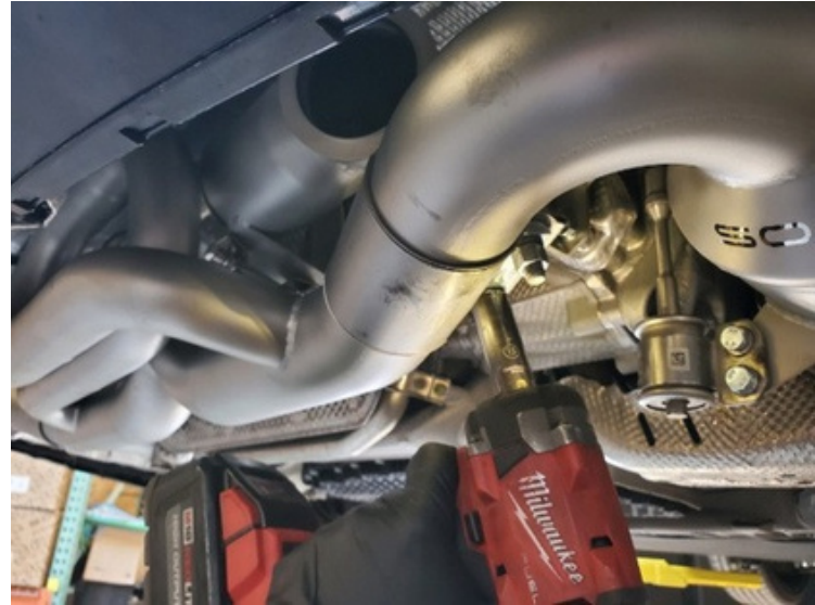
Step 49: Fully Tighten the clamps onto the turbos with a 6mm Allen socket
