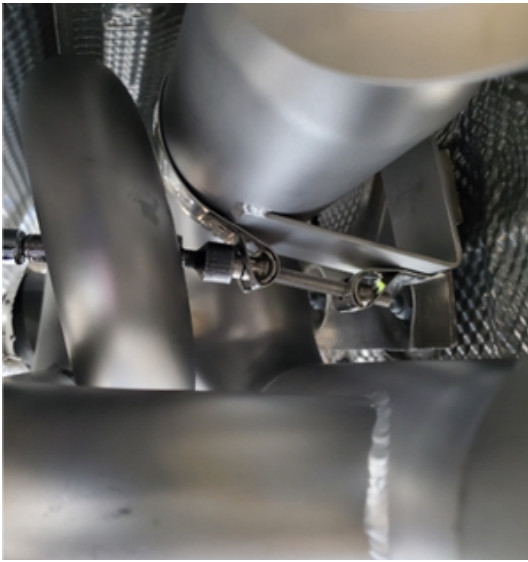
Step 48: Fully Tighten the Torca clamps next with a 15mm Socket.
