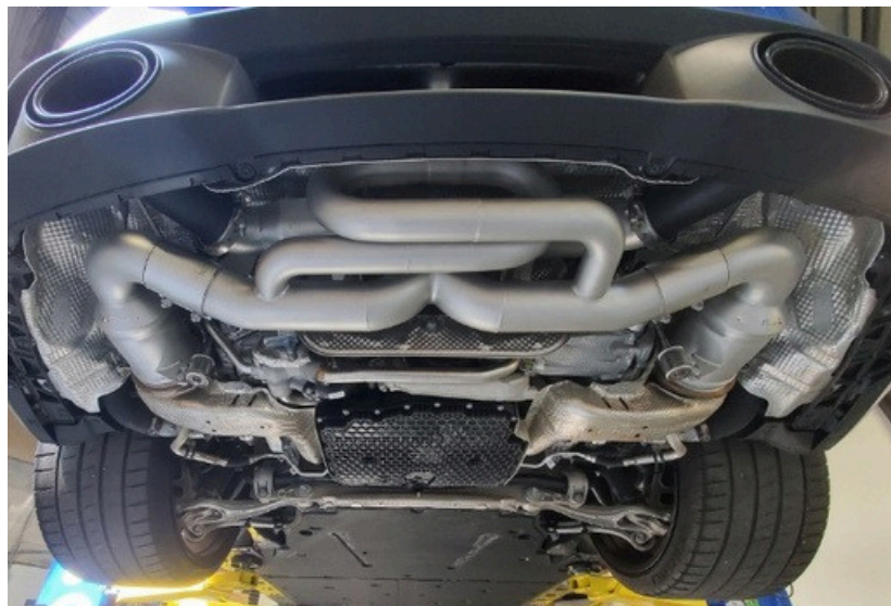
Step 50: Tighten the brackets on the cats last with a 13mm socket and wrench
