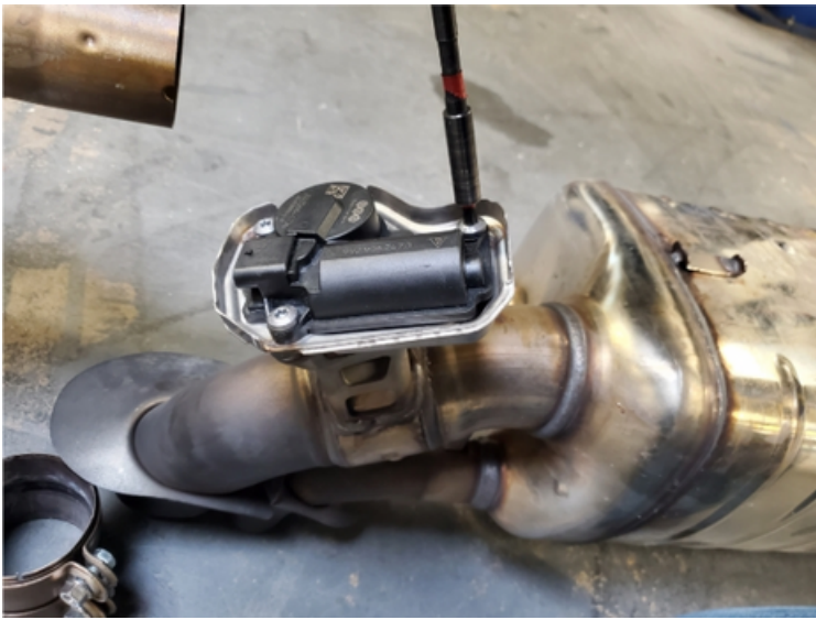
Step 16: You will re-use the Valve motor, and the (6) bolts with the T-30 heads.
