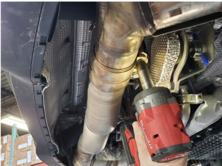
Step 38: Tighten the strap clamps around the resonators on the X-Pipe first.(13mm)
