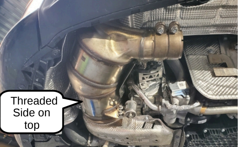
Step 27: Pre-place the clamps onto the catalytic converters. Have the threaded part of the clamp on the top for easier access. Install and tighten the O2 sensor(22mm) while you lift it in place. Only Install (1) Converter for now.
