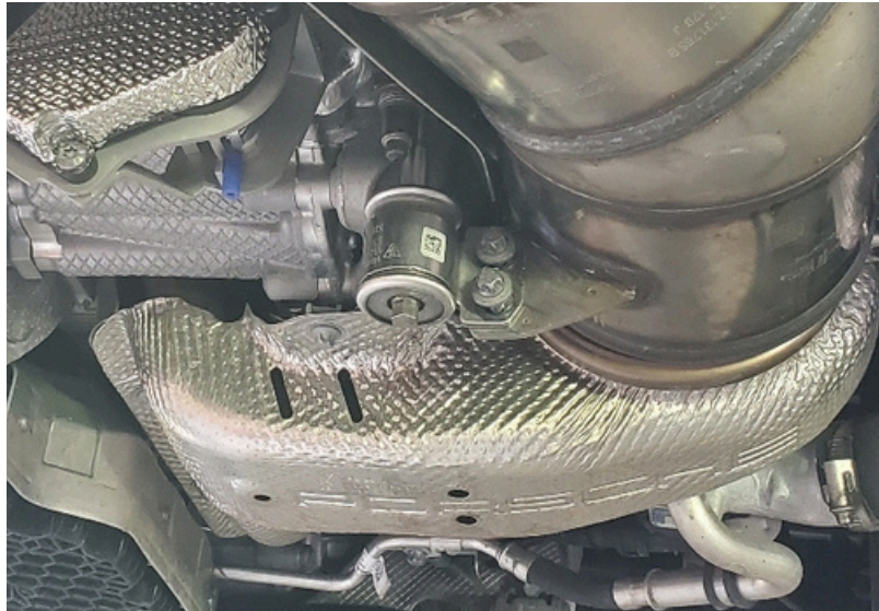
Step 38: Tighten the strap clamps around the resonators on the X-Pipe first.(13mm)
