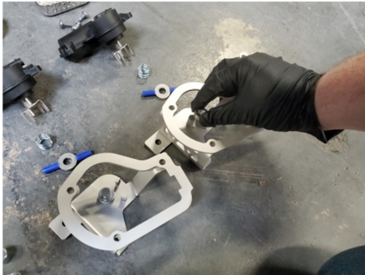
Step 18: Install the "valve position keys" on top of the spacers.
