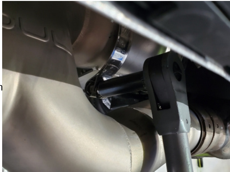
Step 39: Next tighten the clamps between the Cats and Pipe.(13mm)
