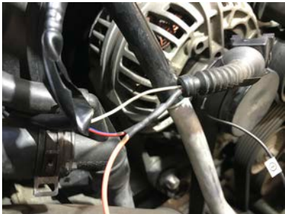
Step 23: Pull 12V key hot power from this solenoid.
