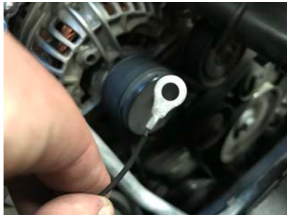
Step 24: Add included eyelet to ground wire and ground to the first runner.
