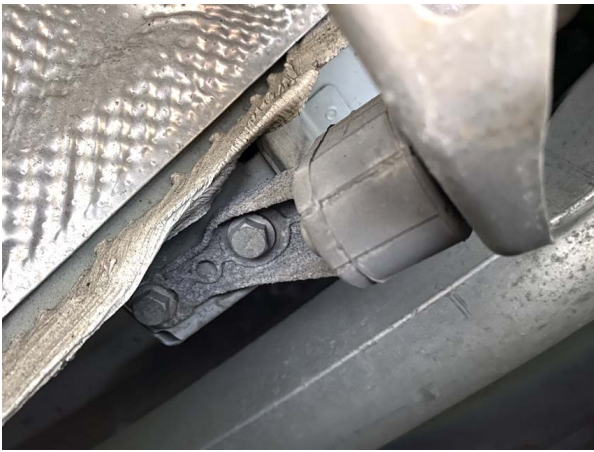
Pictured Right: Carefully remove rear exhaust from vehicle.
